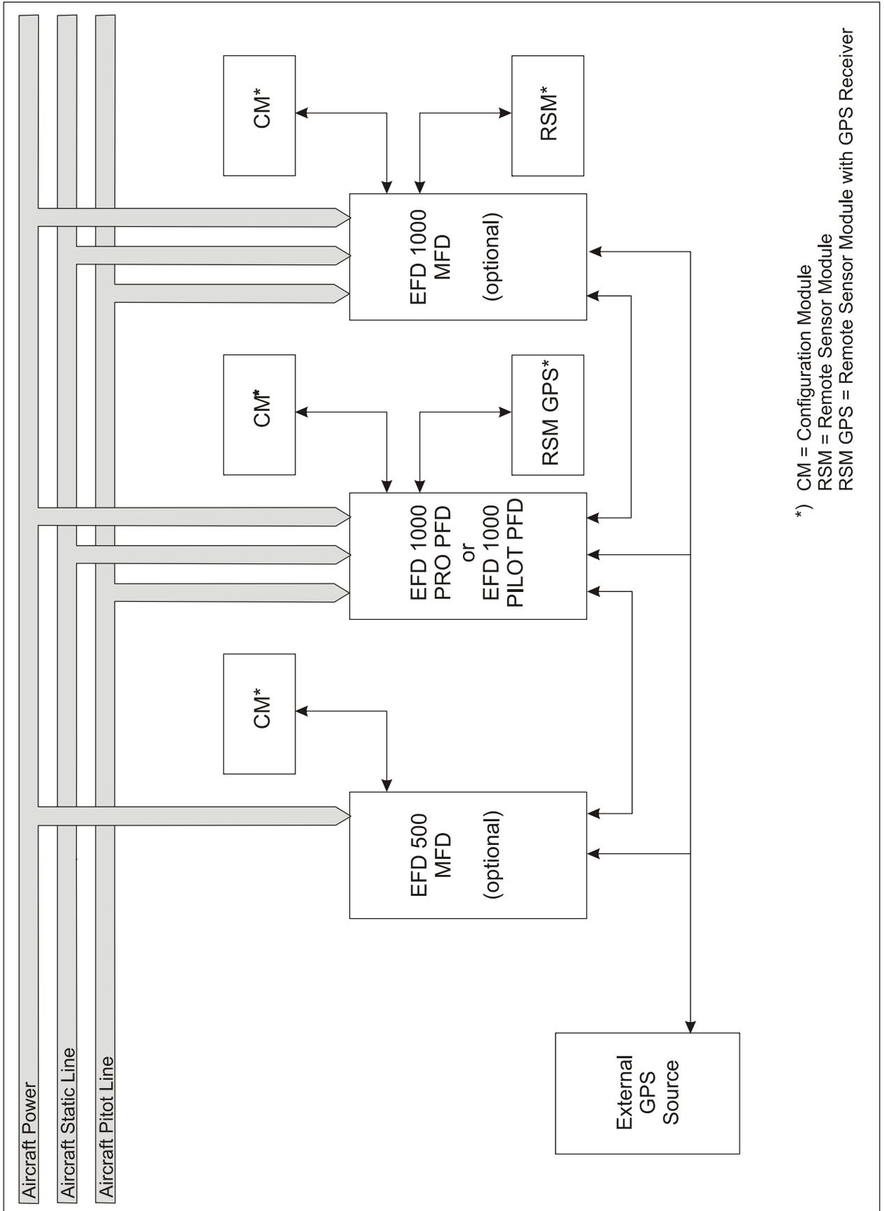
Figure 1, Equipment Configuration
