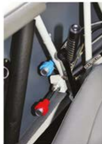
Throttle (black lever), mixture & prop
