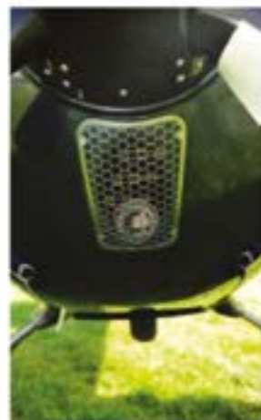
Tightly cowled, the Lycoming can be a b****r to hot-start
