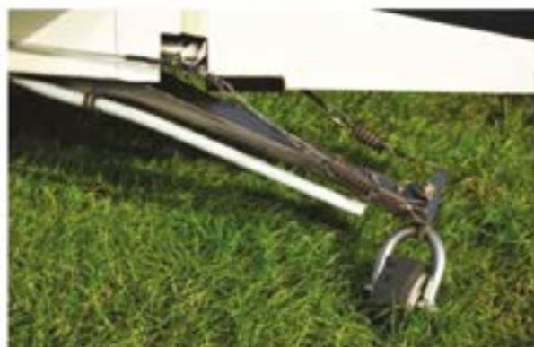
Tailwheel has a carbon-fibre spring and is set well back
