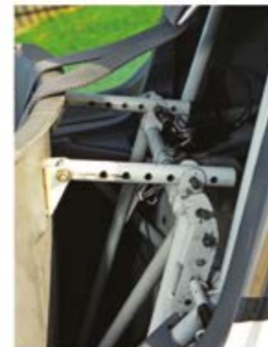
Rear seat, at least, is ground adjustable
