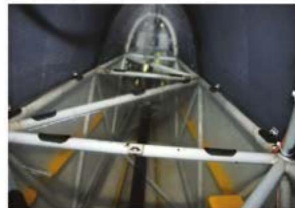
The 330LX is the last in the line to have a steel-tube fuselage
